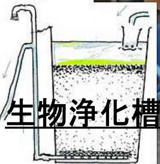
Under drainage porous pipe covered with mesh cloth.
